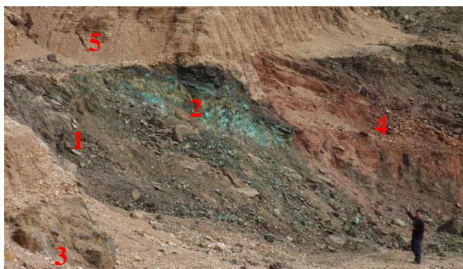
Figure 23: The northern side of open pit "J": (1) Sandy lithofacies; (2) Shaly lithofacies rich with veins of copper silicates; (3) Relict of dolomitic lithofacies; (4) Shehoret Fm. red sandstone with lateral transition to the top Sasgon Mbr. and (5) Alluvium sediments.
