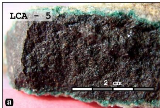
Figure 21: A hand specimen of a Cu-sulphide concretion (dark gray) from the Lower Cretaceous sandstone. Note that the green rim consists of malachite and paratacamite minerals replacing the Cu-sulphide minerals (from Asael et al., 2012).
